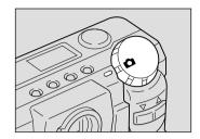
2 Press the Flash button to select the flash mode ( • 4 • 4 Light • 4 Blink).
